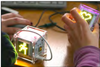
Figure 1: The ConnectUs toolkit, comprising of interactive sensing cubes with Bluetooth connectivity
